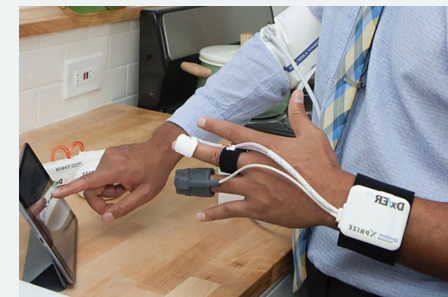
(Above and Below) The DxtER was designed to parallel the Star Trek diagnostic tool, the tricoder, and can identify 34 diseases including pneumonia, stroke and diabetes through the use of a tablet that is connected to a suite of Bluetooth sensors.
