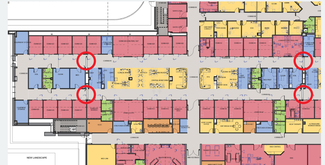
Many hospitals divide their EDs into multiple compartments based on acuity level, providing fire doors, typically on hold opens between compartments. By closing their fire doors, any facility can create subcompartments within the ED. Image of Banner - University Medical Center Phoenix ED Expansion. HKS, Inc.
